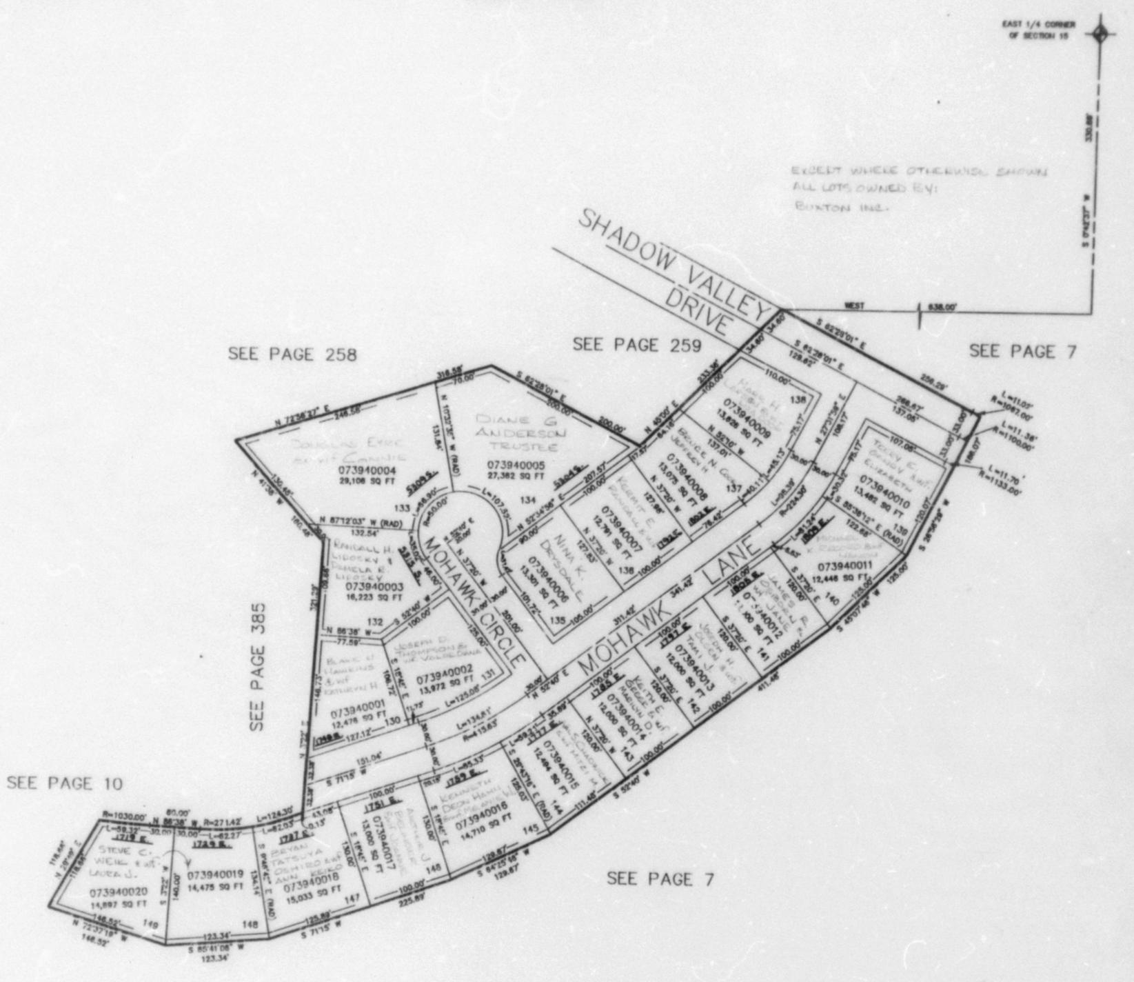
7' UTILITY & DRAINAGE EASEMENTS EACH SIDE OF PROPERTY LINES AS INDICATED BY DASHED LINES EXCEPT AS OTHERWISE SHOWN.
